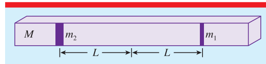
Figure 3. Black box with two unequal masses ( m_1 and m_2 ) placed at equal distances L from the midpoint of the box.
