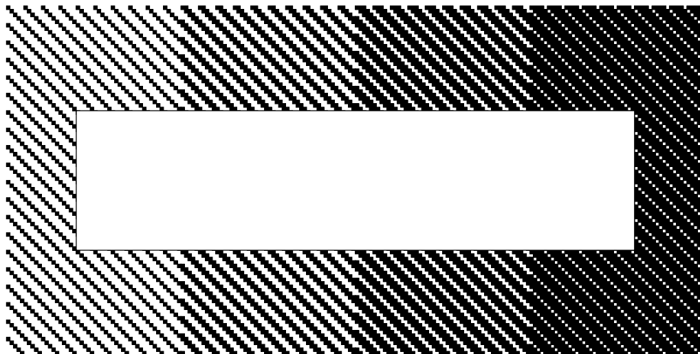
Figure 7.4: Ringelmann grid for smoke density estimation.
